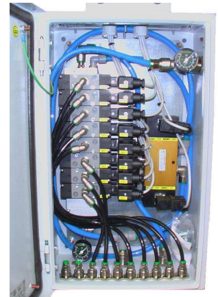
EP SWITCHBOARD WITH ELECTRIC DRAINAGE
